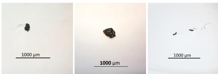
Figure 26. Black particles isolated from oysters from Pula Harbour (samples MAG 41, 10 and 5).
