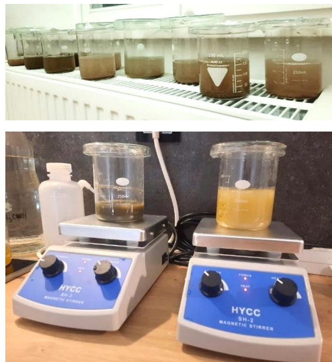
Figure 20. Heating of samples on a radiator (top) and on a magnetic stirrer (bottom).
